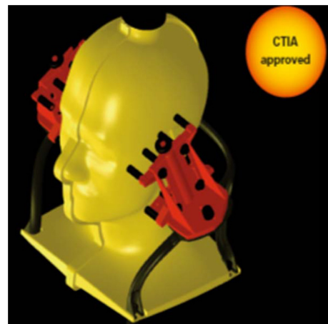
Fig. 2. SAM Phantom. The red devices are clamps to hold the cellphone in a specified location. “CTIA” is the Cellular Telecommunications Industry Association. Source: Speag Phantom Product Flyer.
